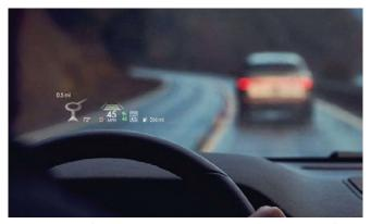
Highly useful vehicle system and driving info is shown right in front of the driver, on the windshield in the available head-up display.2
