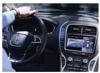
Onboard cameras present the driver with an available 360-degree view of the vehicle's surroundings. This is a Nautilus interior image.
